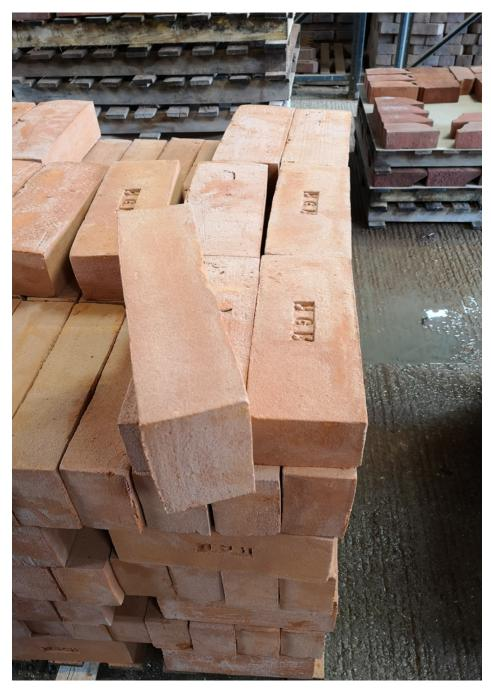
These are shoulder bricks that are specially made to be used for carvings. The clay is put into liquid form before drying.
