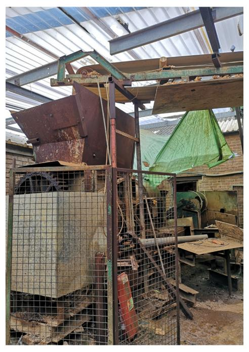
Excess clay is brought to this bucket which can later be fed back into the main clay bed mound.
