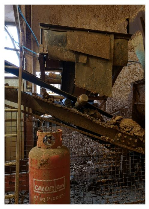
First conveyor belt bringing the clay to the rollers.
