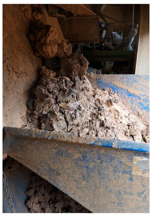
Where the fresh clay is dumped to be transferred on the conveyor belt to be taken through the rollers.
