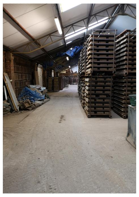
Entrance to the main brick making area where skids are being set and drawn into the drying rooms.
