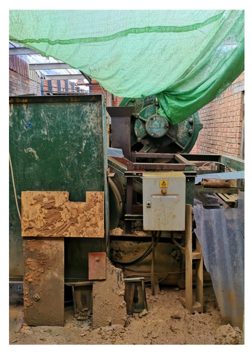
Equipment behind the kilns collecting the rubble from the rollers.
