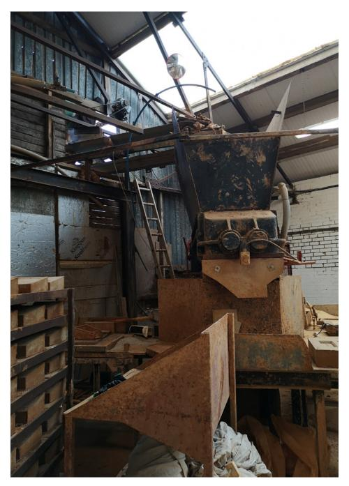
A lot of clay gets stuck in the conveyor belt because it is so sticky which can cause a lot of hiccups in the work unless taken care of.
