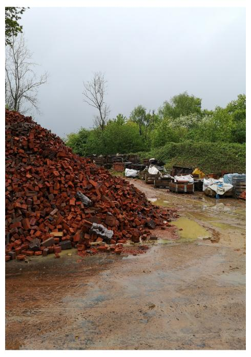
Broken bricks that come out of the kiln can be crushed down and put back into the mixture.
