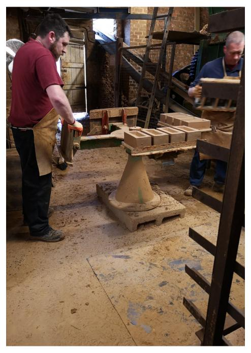
Workers remove the moulds and send them back into the machine to continue the process.
