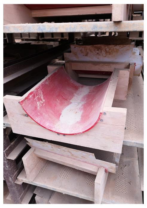
Moulds used for Ridge tiles for roofs. They are made out of rubber and wood.
