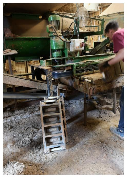
There are two extra moulds laying beside because the other 14 circulating in the machine need to be power-washed every hour.
