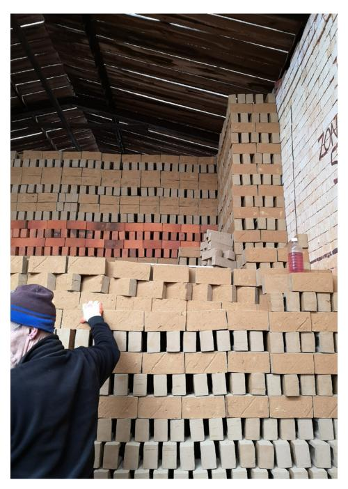
Bricks have to be dry enough to be able to be stacked and not crushed in the kilns.
