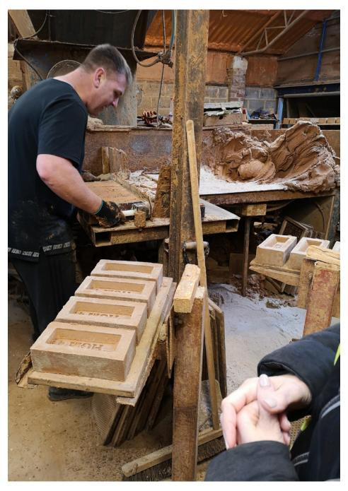
Clay is pumped up to the working bench where they roll clumps of clay into the sand and dust their moulds with sand.
