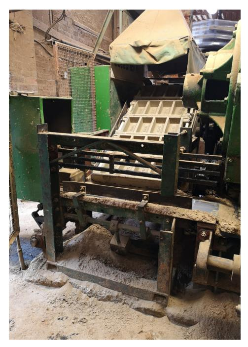
Better view of the moulds after being dusted with sand.
