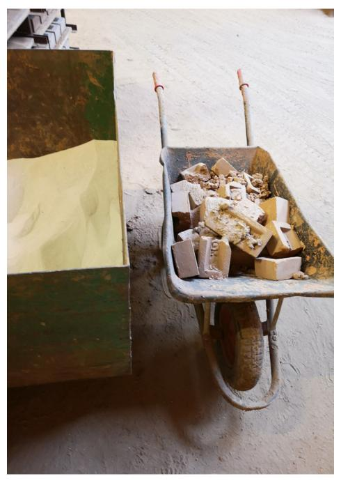
This is the sand that is dusted on all the moulds to allow the clay to slip easily away without damaging the bricks.
