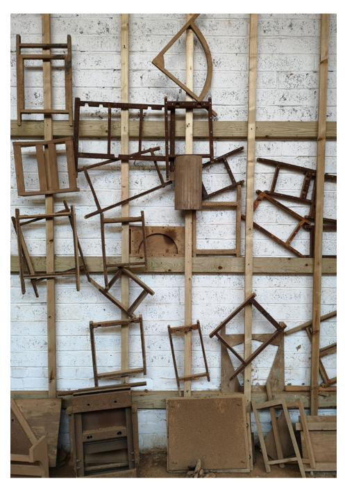
Moulds used to make roof tiles are all done with slip-mould method.
