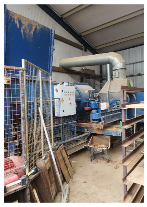
This is the machine used to mix the clay with straw to create the Strocks.
