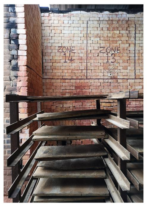
In the oil kilns, there are 14 tunnels which is where the fire is located to move the heat around the kiln.
