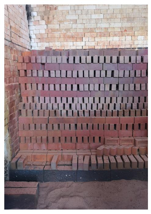
Stacking the bricks to be in the right order and to create and arch around each tunnel is an art in itself.
